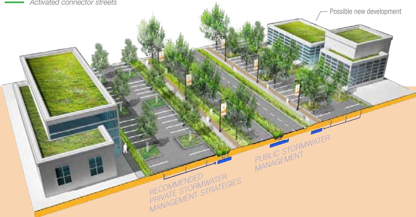
Proposed upgrades to Essington Avenue including multimodal accessibility, as well as private and public stormwater management systems
