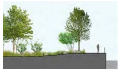
Typical trail section at river bulkhead, with 100' development setback that serves as functioning green stormwater element while creating needed open space along the river
