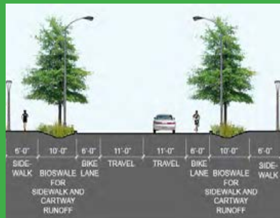
Typical bioswales collecting runoff from streets and sidewalks
